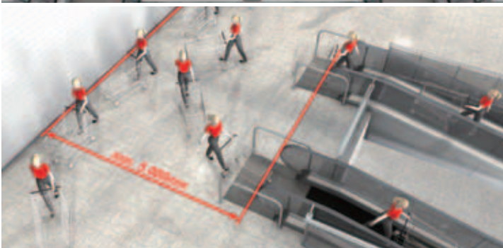
min. 400 mm, otherwise wedging guard required
