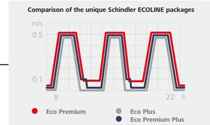
Frequency converters for up to three different speeds.
